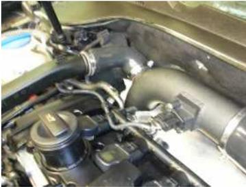
Step 7: Start up the car and listen for any leaks, take the car for a test drive, and then retighten all clamps just to be safe. \*Tip\* to test for leaks spray some soapy water on all the silicone connections, if it bubbles, you have a leak. Enjoy!
