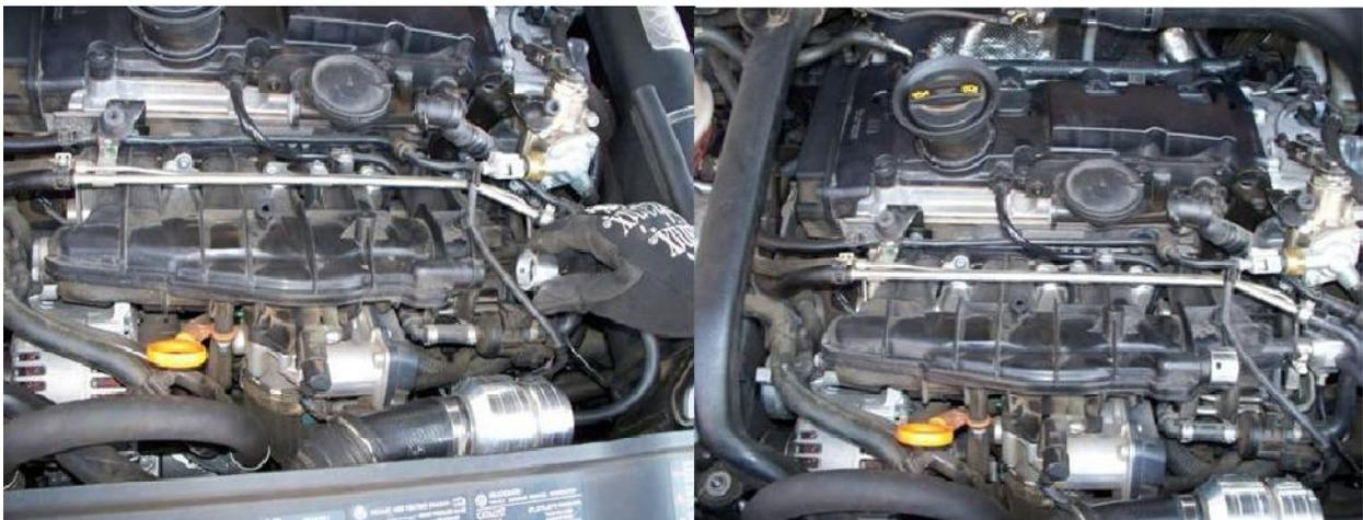
**Step 3:** Remove the front PCV assembly. Start by removing the hose on the driver side. The clip that holds it in place has 4 teeth. Remove the side teeth and the top tooth by gently lifting them up and over the lip on the nipple one at a time with your flat head screwdriver. When those are
