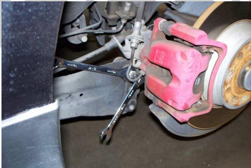
**Step Three:** Using the same method as step two unbolt the factory end link from the swaybar. Once the nut is removed use your triple square to unthread the end link from the swaybar. Remove the end link from the vehicle.
