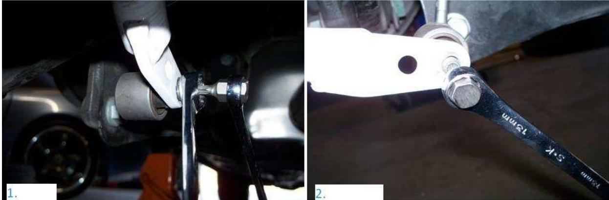
**Step Four:** Install BSH End Link per the image below. The bolt heads should be resting on the side of the bearings with the retaining clips. The spacers should be against the sides with more billet material covering the bearings. The BSH logo should be facing in on both sides of the vehicle.
